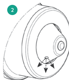
The residual pressure is released by the small holes during connection
